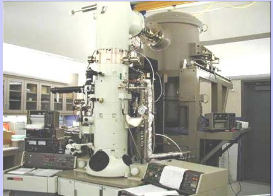
JEOL FEG 300 kV, liquid helium-cooled
